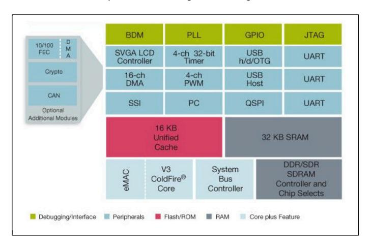
View additional information for ColdFire® V3 Microprocessor with LCD driver, Ethernet, USB and CAN.
