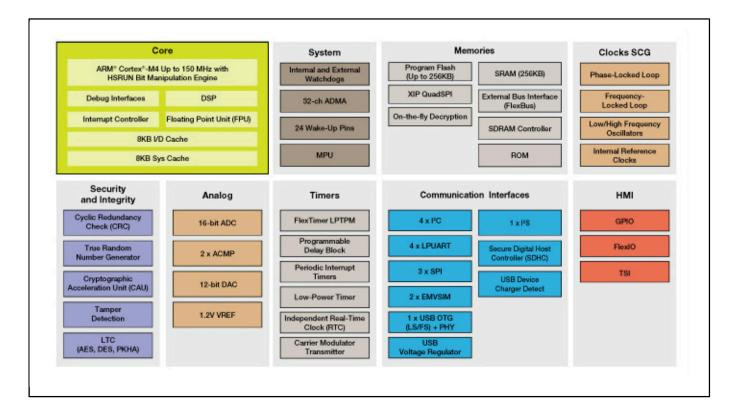
View additional information for Kinetis K81-150 MHz HW Cryptographic Co-Processor, Anti-Tamper and QuadSPI Microcontrollers (MCUs) Based on Arm® Cortex®-M4 Core.
