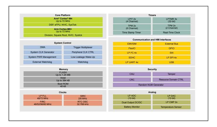
View additional information for NXP's Energy Efficient Cortex-M4 MCU with Cortex-M0+ and Advanced Security.
