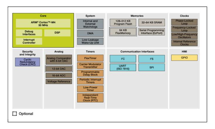
View additional information for Kinetis® K12-50 MHz, Microcontrollers (MCUs) with Optimized Features based on Arm® Cortex®-M4 Core.
