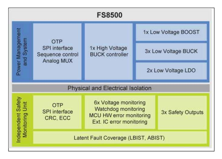
View additional information for Safety System Basis Chip for S32 Microcontrollers, Fit for ASIL D.
