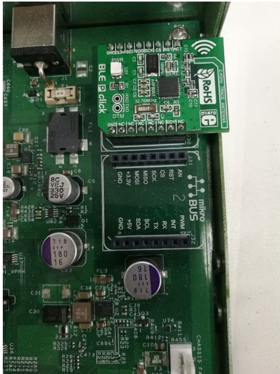
Figure 61. BLE P click board hardware setup
