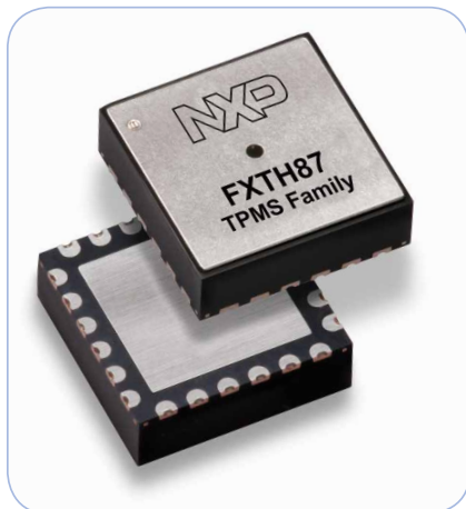
Figure 5: Standard TPMS packages include 7 x 7-mm QFN.
