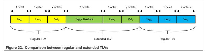
Figure 32 illustrates the comparison between regular and extended TLVs.
