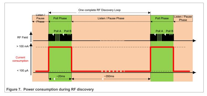
In a typical set-up, the polling phase is approximately 50 ms long while the listening phase is approximately 350 ms long (this set-up is configured thanks to the NCI parameter called TOTAL\_DURATION).
