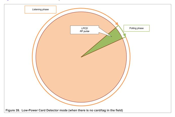
Figure 39 illustrates the RF Discovery when the LPCD is enabled.
