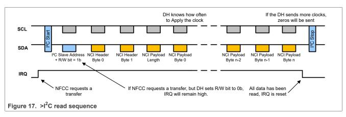
Figure 17 is an example where the IRQ is raised so the DH can proceed a read.
