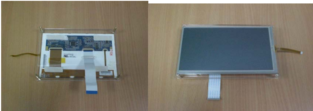
Figure 2-8 Attach the LCD to the Panel
