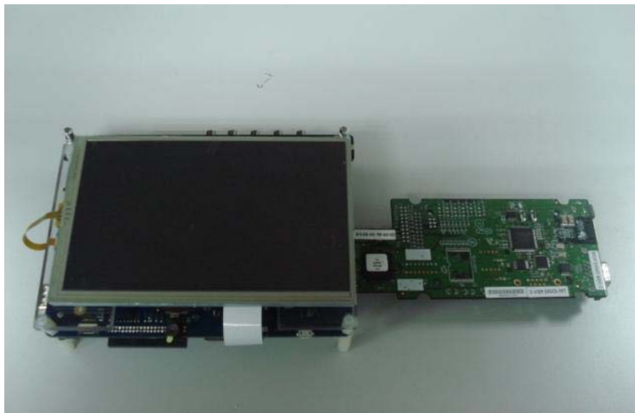
Figure 2-9 Attach the LCD to the Personality Board
