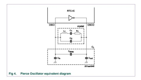
The inverting amplifier (with feedback resistor, and drive resistor which are not included in Fig 4) is incorporated within the integrated circuit device. On the other hand, the quartz crystal is a discrete device external to the integrated circuit. In the PCF85x3, PCA8565 and PCF2123, PCA21125 the output capacitor Cout is integrated on the integrated circuit. PCF8563A, PCA8565A and PCF2123 also include Cin, see Table 3 for overview.
