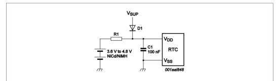
(1) Due to the low RTC current consumption, a parallel diode over  $R_1$  (directed from the battery to the RTC) will not be of any use. The voltage drop over  $R_1$  is small
