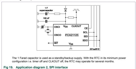
**Remark**: CLKOUT and INT are open drain outputs. If a pull-up resistor is used, it should not be connected to voltages higher than the maximum operating voltage as specified for the RTC. If the outputs need to be used to switch signals connected to a higher potential, it is necessary to use an external transistor.
