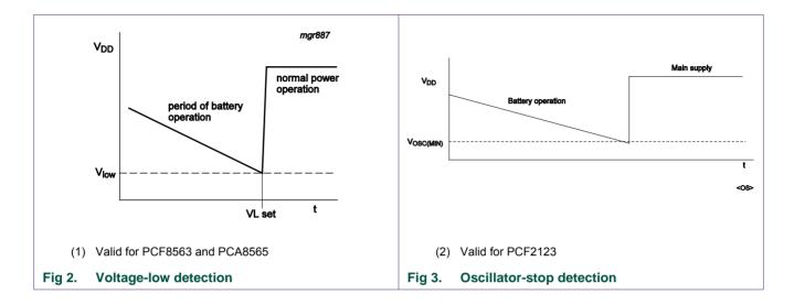
In the case of PCF8563/PCA8565 bit VL set indicates that the integrity of the clock information is no longer guaranteed. If the oscillator hasn't stopped, the clock information will still be ok, but with  $V_{DD}$  having dropped below  $V_{low}$  there is no guarantee that this still is the case because there is no way to be sure that the oscillator kept running. The VL flag can only be cleared by software.
