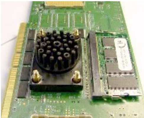
Figure 7-13. Allen screws removed
