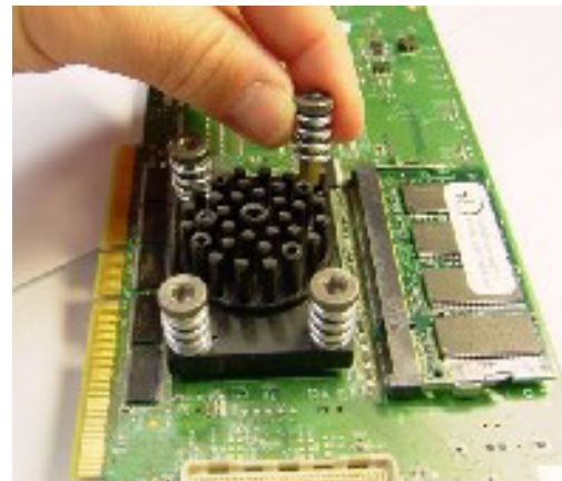
Figure 7-12. Remove Allen screws by hand
