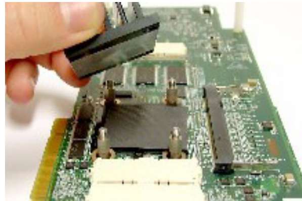
Figure 7-14. Remove heat sink
