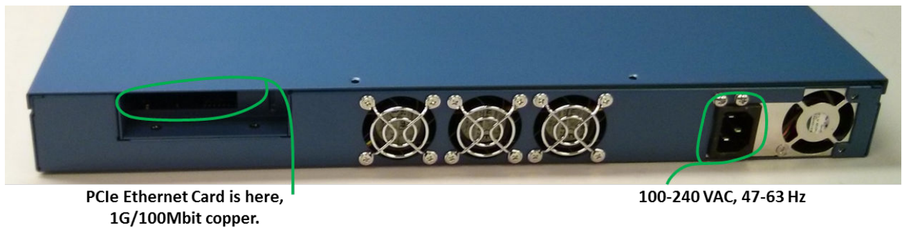
Figure 5. LS2085ARDB/LS2088ARDB rear panel
