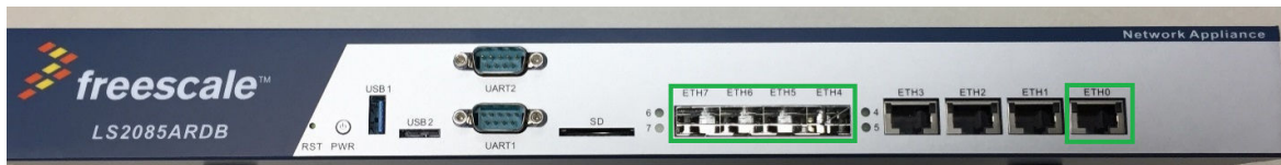
Figure 4. LS2085ARDB/LS2088ARDB front panel
