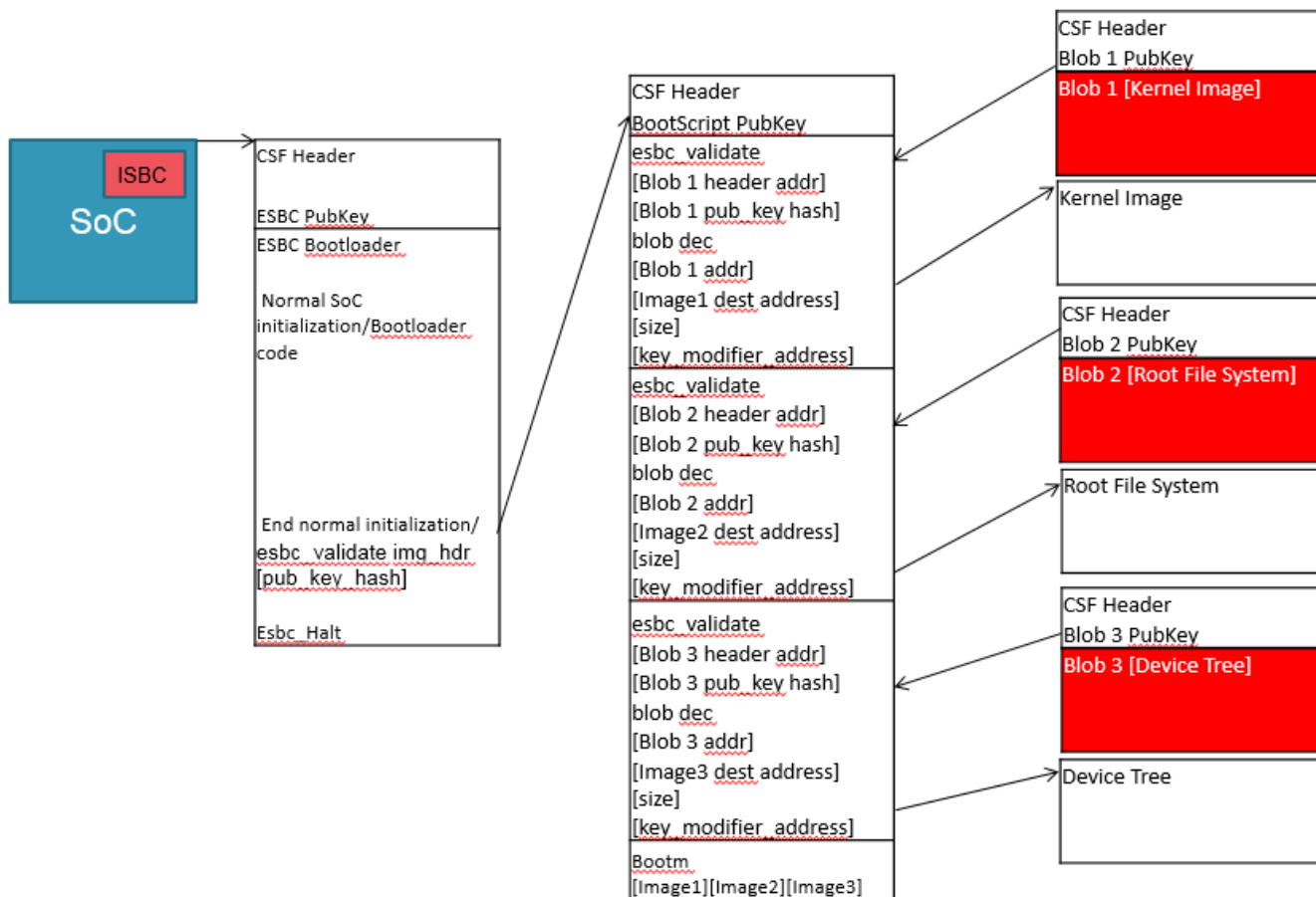
Figure 317. Chain of Trust with Confidentiality (Decapsulation)
