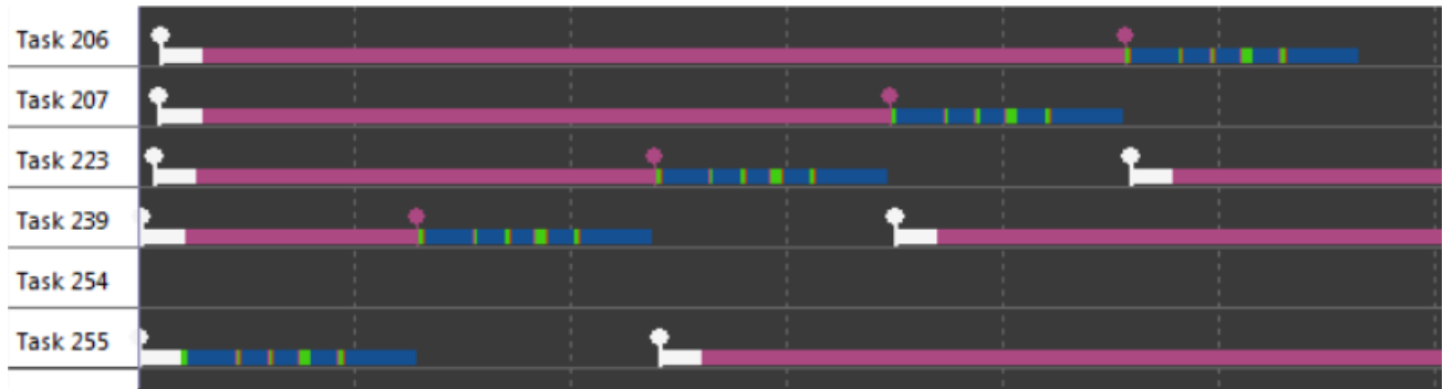
Figure 53. Tasks Executing Sequentially
