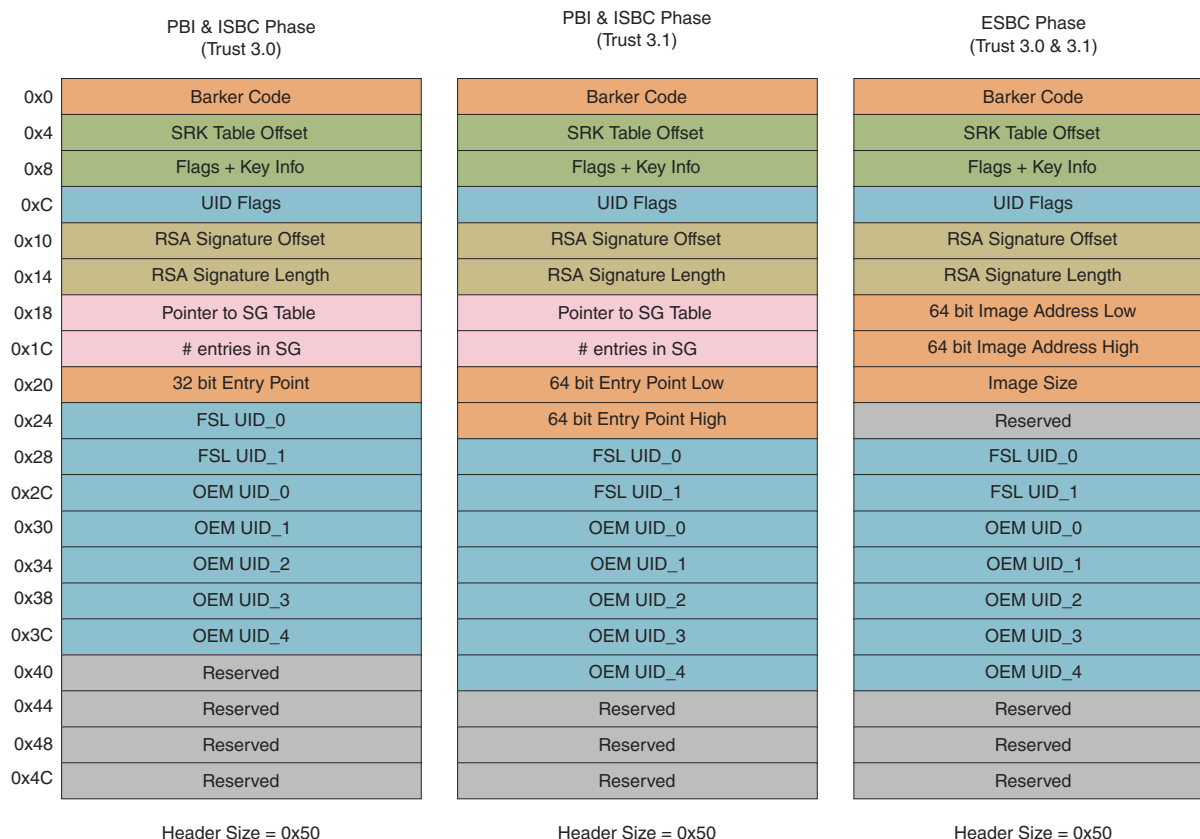
Figure 340. CSF Header Structure
