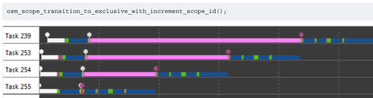
Figure 55. Tasks in a Flow Blocking for Exclusivity
