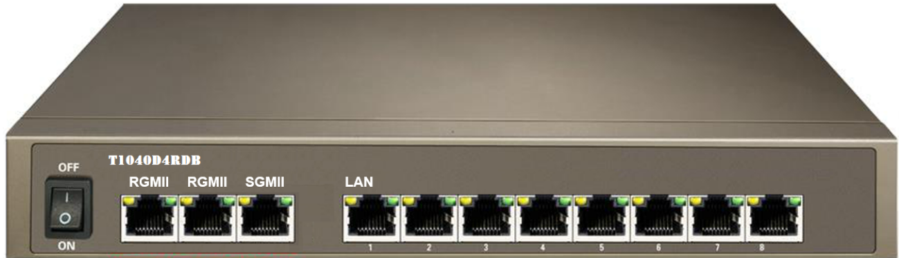
Figure 216. T1040D4RDB WAN ports and LAN ports
