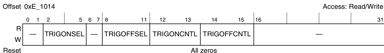
Figure 20-5. Performance Monitor Local Control Register B0 (PMLCB0)
