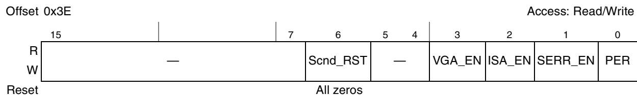
Figure 18-77. PCI Express Bridge Control Register
