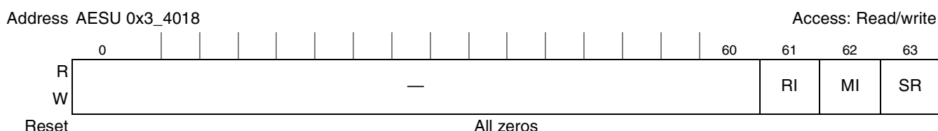
Figure 12-50. AESU Reset Control Register
