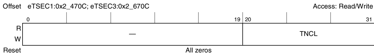
Figure 15-87. Transmit Total Collision Counter Register Definition
