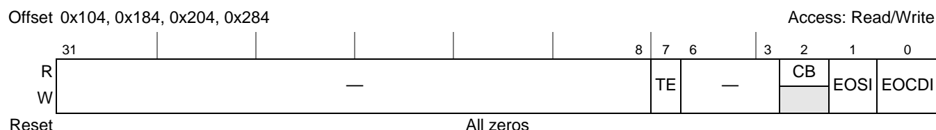
Figure 14-3. DMA Status Register (DMASR n )
