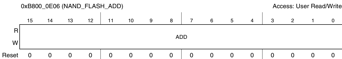
Figure 20-6. NAND Flash Address Register
