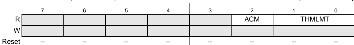
Figure 25-16. Driver Amplifier Control Register (IIM_DRVACR)
