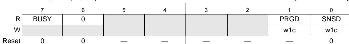
Figure 25-2. IIM Status Register (IIM_SR)
