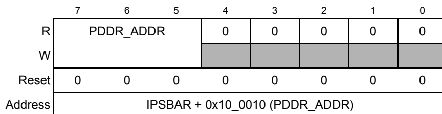
Figure 12-12. Port ADDR Data Direction Register (PDDR_ADDR)
