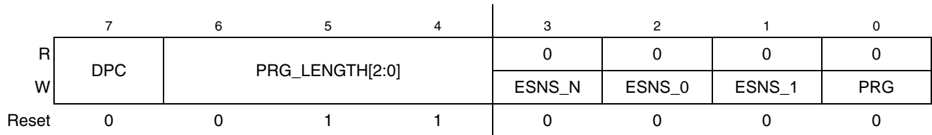
Figure 29-7. Fuse Control Register
