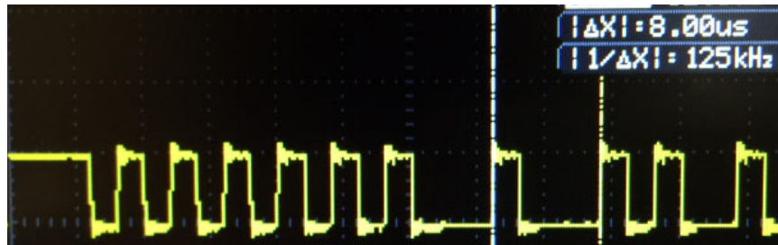
Figure 13. TxD pin at start of CAN 2.0 transmit frame with standard ID 0x555
