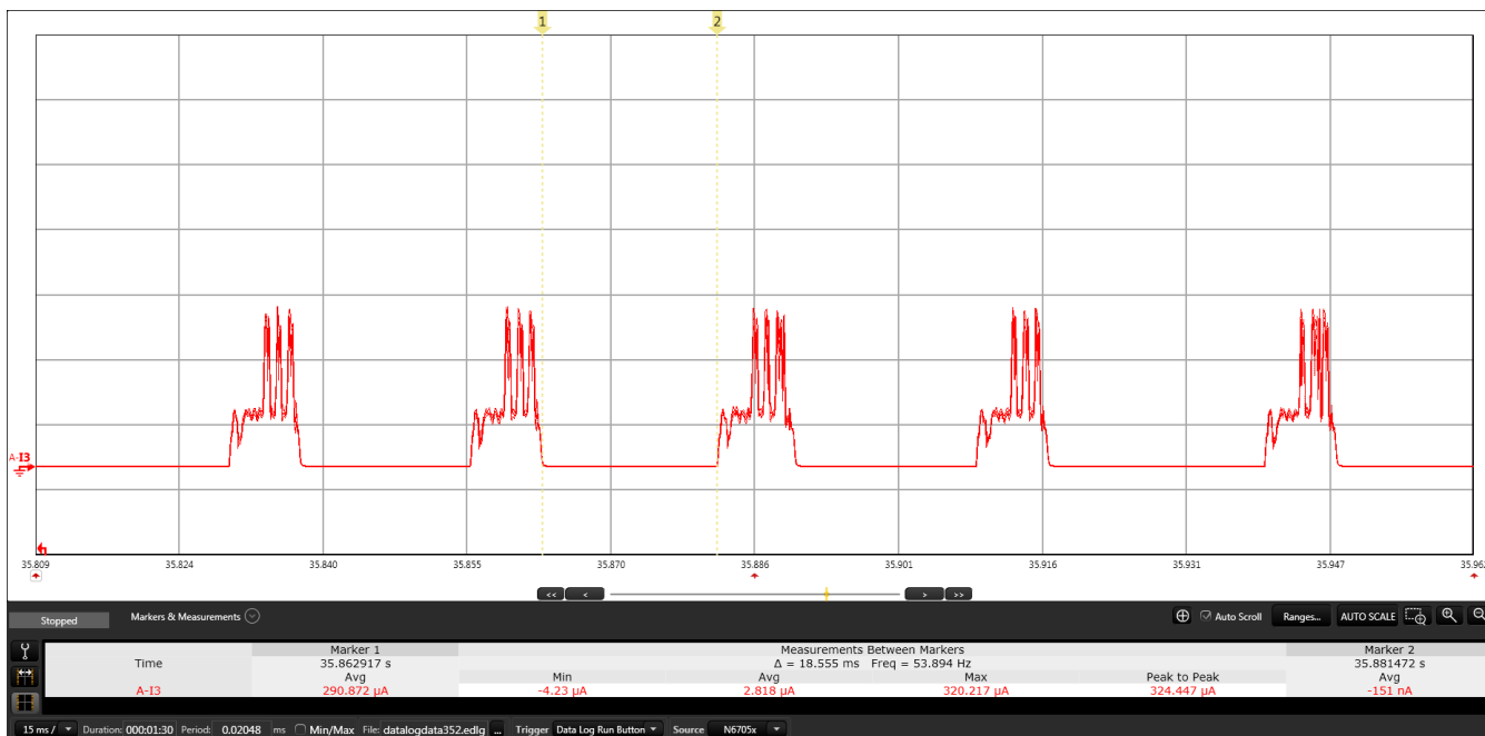
Figure 22. Current consumption in low-power mode 1 (fast ADV)
