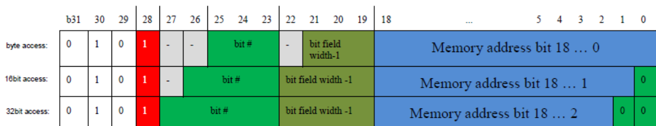
Figure 3. Address bits for bit field insert/extract operation
