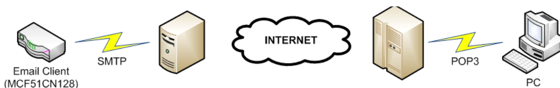
Figure 1. Email client connecting to an SMTP server
