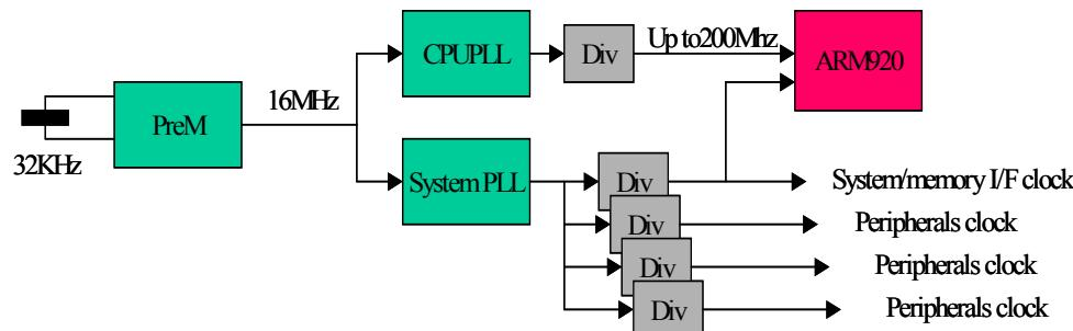
**Figure 1. System Clocking Scheme**
