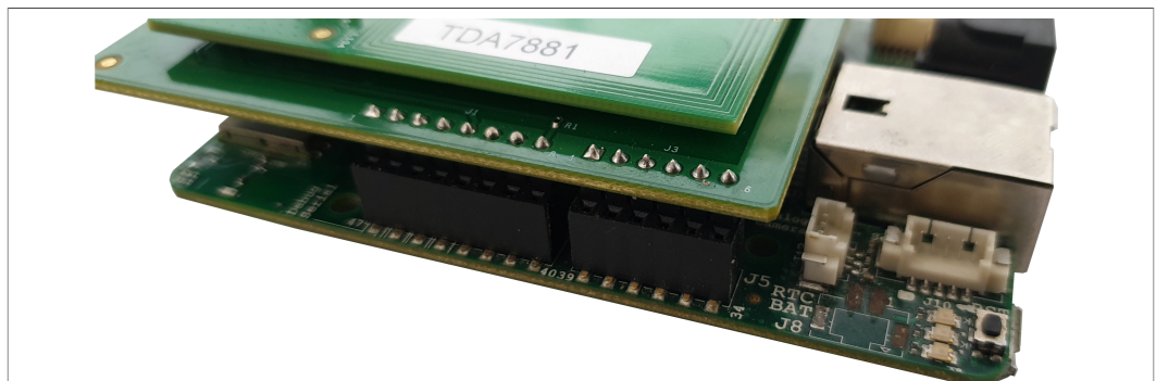
Figure 4. OM5579/PN7150ARD and UDOO Neo stacked together - zoom
