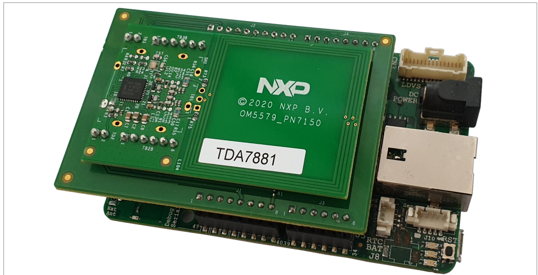
Figure 3. OM5579/PN7150ARD and UDOO Neo stacked together
