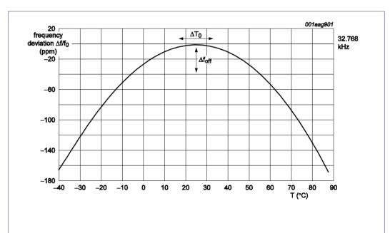
Fig 1. The deviation of frequency w.r.t. temperature of a typical 32.768 kHz crystal
