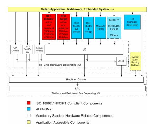
Just to clarify: The components of "RF Chip Hardware Depending I/O" and "Platform and Peripheral Bus Depending I/O" have to be included in any of all possible solutions.
