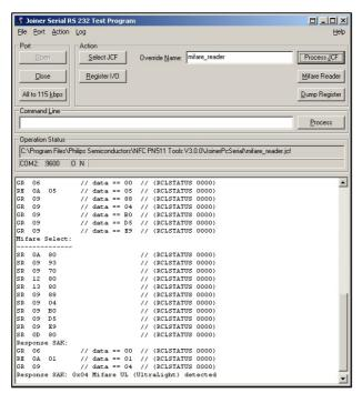
Scrolling down to the end of the trace window the Select Acknowledge (SAK) can be read off. For this example with the MIFARE® UL card it has to be 0x04. If the MIFARE® Classic 1k is placed on the antenna the SAK is supposed to be 0x08.
