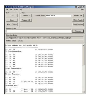
The first line sets register 01 with value 0x0F. A soft reset is performed. The status variable RCLSTATUS showing 0 indicates that no error in the communication has occurred.
