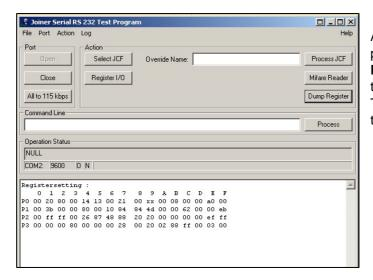
An additional check can be performed using the **Dump Register** button. It returns the actual PN51x settings. The result can be read off in the trace window.
