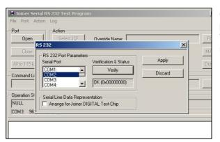
Choose the appropriate RS232 COM port for your serial communication, **Verify** (checks if the port is used or not) your selection and press **Apply**.
