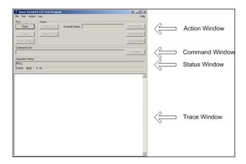
The Joiner Serial RS232 Test Program (=JoinerPCSerial) is a simple User Interface (UI) utility for register-based access to the Joiner hardware using the serial interface and the Basic Function Library (BFL).
