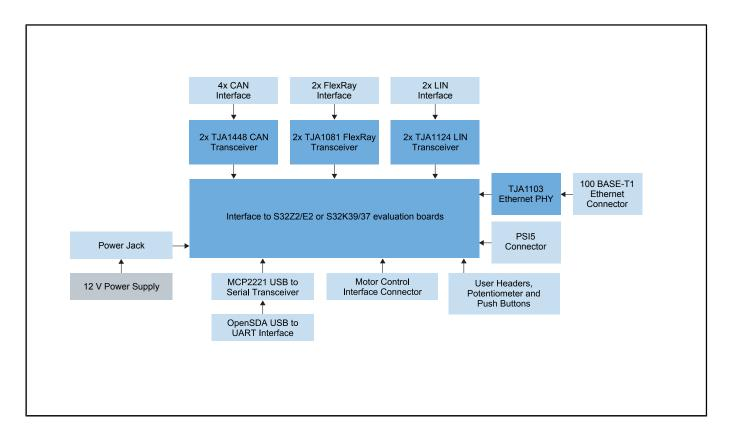
View additional information for S32X-MB I/O Extension Evaluation Board for Real-Time Domain Control and Actuation.
