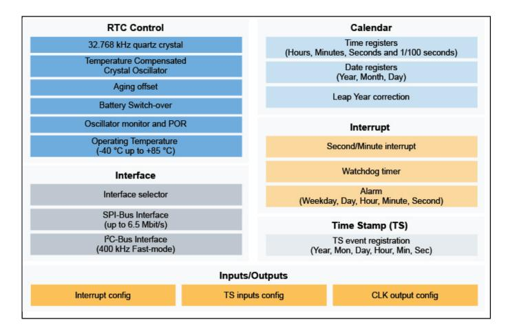
View additional information for Nano-Power Highly Accurate RTC with Integrated Quartz Crystal.
