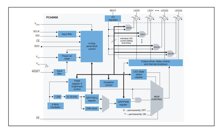
View additional information for PCA9958 24-Bit 63 mA Current LED Driver with SPI.
