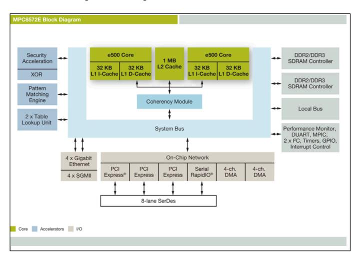
View additional information for PowerQUICC® III Processor with DDR2/3, Pattern Matching Engine, PCI Express®.
