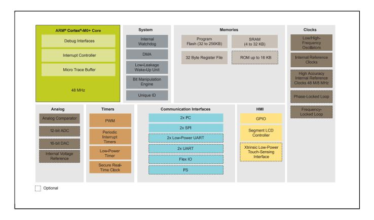
View additional information for Kinetis® KL3x-48 MHz, Segment LCD Ultra-Low-Power Microcontrollers (MCUs) based on Arm® Cortex®-M0+ Core.
