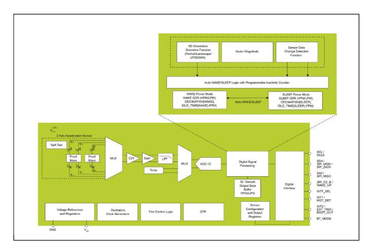
View additional information for ±2g/±4g/±8g/±16g, Low Power 12-bit Digital Accelerometer.
